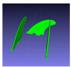
of surfboard and fin shape have been performed. In this project, we want to study the fluid dynamics for surfboard-fins with varying sizes and the influence towards resulting drag and lift forces for different angles of fluid attack and fluid velocities. The question to answer is: Does fin size really have significant influence on forces and if yes where do they affect most forces?
